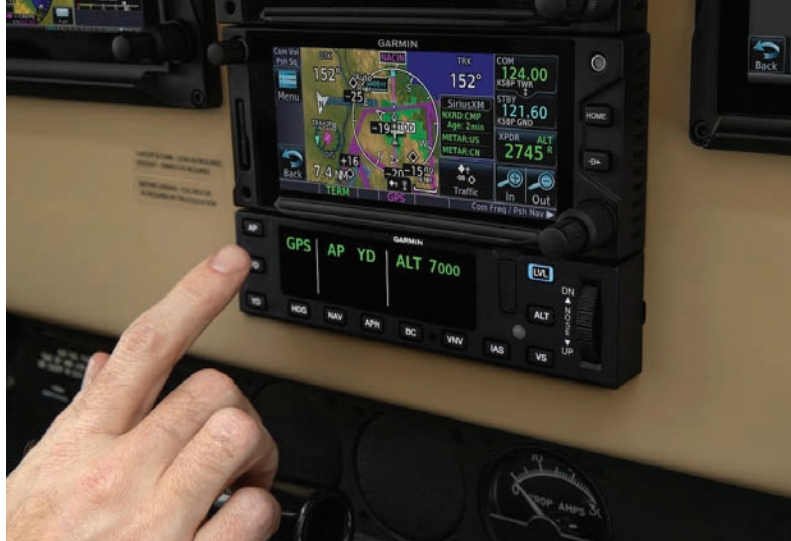
A general aviation autopilot system. (Garmin photo)
