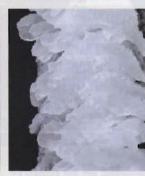
Stills from a NASA video showing the accretion of ice on the leading edge of a wing. Pilots need to reexamine their views if they think that Flight Into Known Icing (FIKI) approval makes their plane impervious to ice. Icing can overpower even good systems and, moreover, many parts of our planes remain unprotected despite having certificated FIKI gear.
